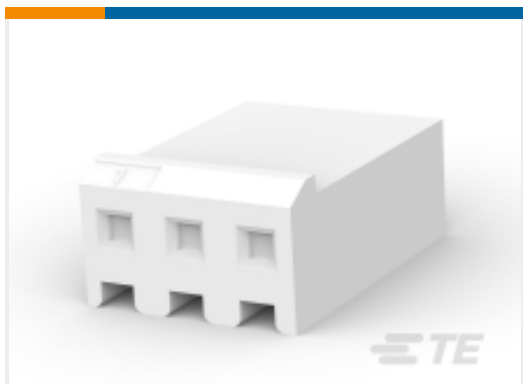
TE Part #1-647402-5 3.96mm Wire-to-board housing: receptacle, with mating alignment, SL 156
