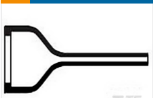
TE Part #808761-000 Heat Shrink Boots: Lipped, Straight
