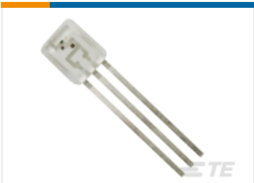
TE Part #11032254-00 PHOTO OPTIC EMITTER ASSEMBLY
