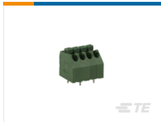
TE Part #1-2834011-4 4POS 3.5MM TOP ENTRY SCREWLESS CONN.
