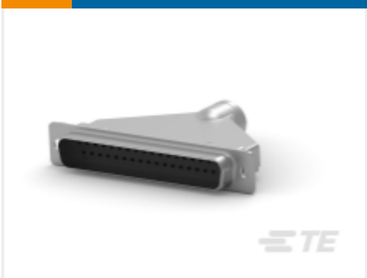
TE Part #205210-8 D-Sub Crimp: Plug, Signal, 37 Posn, Pin Size 20, Shell Size 4
