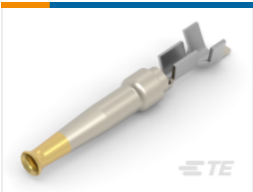
TE Part #1-66504-0 D-Sub Conn Contacts: Socket, Phosphor Bronze, Signal, Size 20
