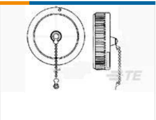
TE Part #211903-1 CMC DUST CAP ASSM SIZE 22
