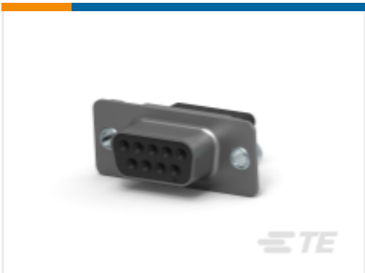
TE Part #1658654-1 D-Sub Crimp Recpt Signal 9 Posn, Socket Size 20, Shell Size 1
