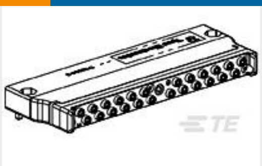
TE Part #1738960-2 CONNECTOR ASY,MODULE,24 POS, ARINC 801
