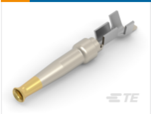
TE Part #1-66505-0 D-Sub Conn Contacts: Socket, Phosphor Bronze, Signal, Size 20
