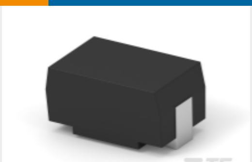
TE Part #3-1879011-7 SMD Power Resistor: 7 Watt, 200-2M Ohm
