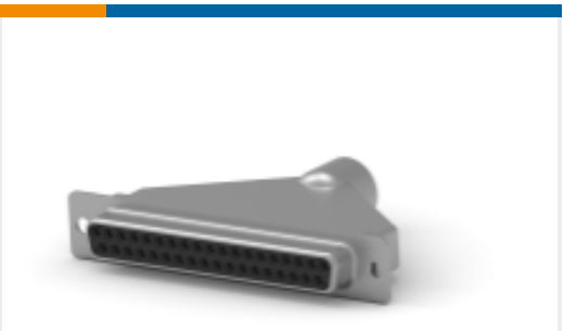
TE Part #1658660-1 D-Sub Crimp Recpt Signal 37 Posn, Socket Size 20, Shell Size 4
