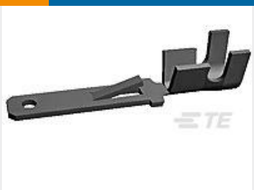
TE Part #170030-2 FF 250 TAB 20-14AWG TPBR
