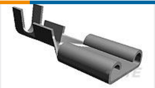
TE Part #42400-1 FASTON 250 TERMINAL REC 18-14 AWG BR
