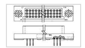
PCB Connector Assembly Type: PCB Mount Receptacle
