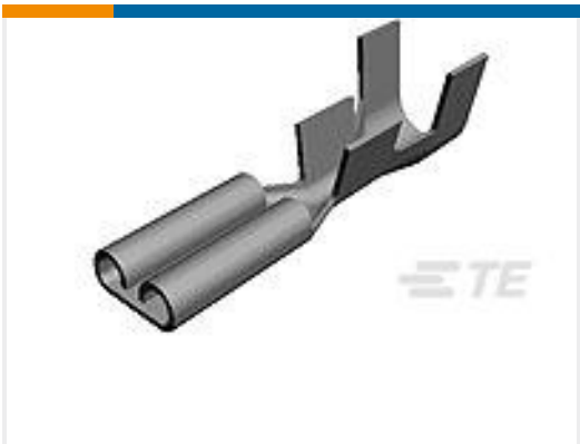
TE Part #170213-2 250 FASTON,REC.,18-14 AWG,TPBR
