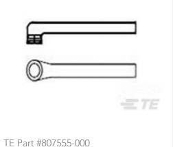
Low Profile Heat Shrink Boots: Poly Mold, Lipped, Right Angle
