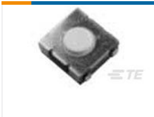
TE Part #1571626-4 TACT,SMT,GULL WING,100GF,T&R
