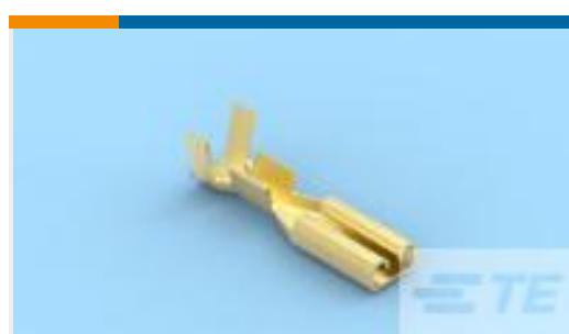
TE Part #881607-1 FASTON 110 REC 0.5-1.0 MM2 0.25 X12.30 BR
