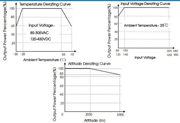
Note: ① With an input voltage between 85-100VAC and a DC input between 120-140VDC the output power must be derated as per the temperature derating curves:
