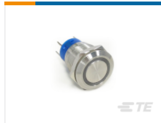
TE Part #1-2213764-5 AV19 SPM 5A FIX RING LED GREEN 24V
