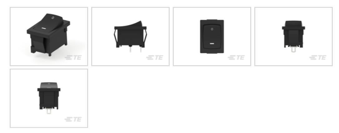
Rocker Switch Type: High Power Rocker Switch Mounting Type: Panel Indicator/Imprint Legend: OI Panel Cutout Size: 13 x 19.2 mm [ .514 x .754 in ] Switch Contact Plating Material: Silver
