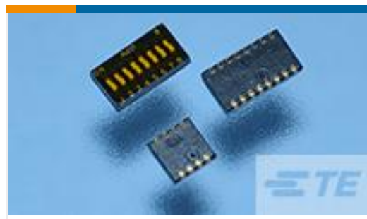
TE Part # 1977831-5 DIP SWITCH GDH10SATR04
