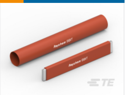
TE Part #419641-000 Busbar Insulation Tubing up to 35 kV
