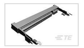
DRAM Type: Double Data Rate (DDR) Stack Height: 5.2 mm [ .205 in ] Module Orientation: Right Angle PCB Mounting Style: Surface Mount Connector System: Cable-to-Board
