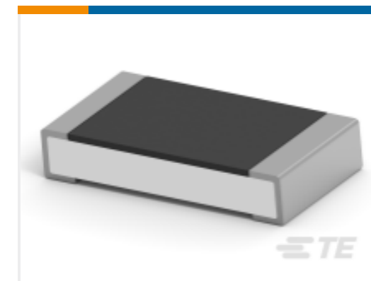
TE Part #1-2176390-2 RQ 1206 1K5 0.1% 10PPM 5K RL
