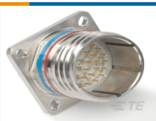
TE Part #YDTS20W15-97BNV001 D38999: Square Flange, 15-97 insert
