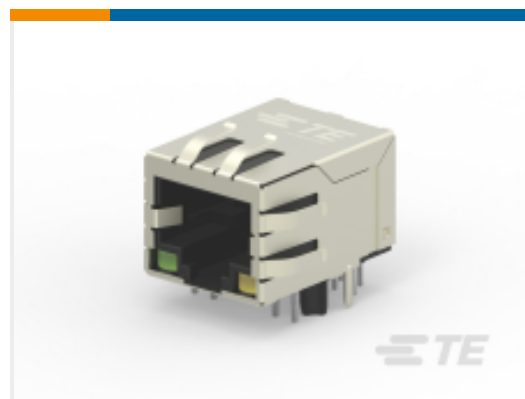
TE Part #1-2301994-2 RJ45 JACK INT.MAG. 1GB LED 1X1
