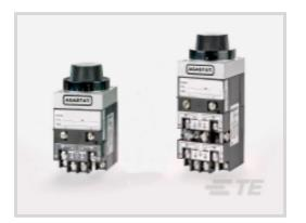
Type of Control: Knob Time Delay Relay Input Voltage: 48 VDC Time Delay Relay Contact Current Rating: 10A@240VAC A Mode of Operation: On-Delay Delay Time: 1 – 300 seconds
