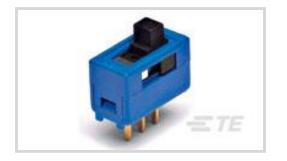
Configuration (Pole-Throw): Double Pole - Four Throw Slide Switch Mounting Angle: Vertical Contact Base Material: Copper Alloy Number of Actuators: Single Number of Slide Switch Positions: 4
