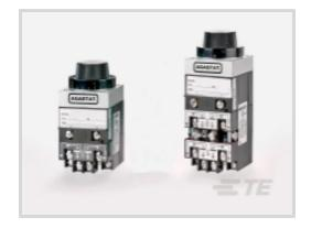
Type of Control: Knob Time Delay Relay Input Voltage: 240 – 220 VAC Time Delay Relay Contact Current Rating: 10A@240VAC A Mode of Operation: On-Delay Delay Time: 3 – 30 minutes
