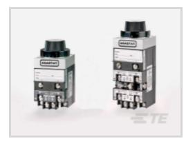
Type of Control: Knob Time Delay Relay Input Voltage: 48 VDC Timing Range (Off-Time): .5 – 5 seconds Time Delay Relay Contact Current Rating: 10A@240VAC A Mode of Operation: Off-Delay
