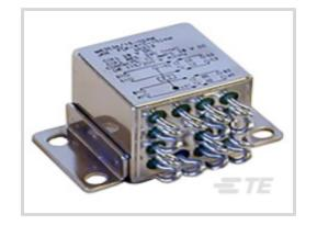
Type of Control: Fixed Time Delay Relay Input Voltage: 28 VDC Time Delay Relay Contact Current Rating: 10A@28VDC A, 115VAC A Mode of Operation: Delay on Release Delay Time: 6 seconds
