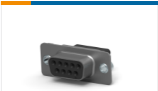
TE Part #1658643-1 D-Sub Crimp Recpt Signal 9 Posn, Socket Size 20, Shell Size 1
