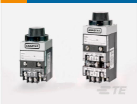
TE Part #7-1423162-5 7022ACX=RLY,STD,OFF,2P,120VAC, 15SEC,X OP
