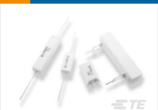
TE Part #1623781-7 Wirewound Resistor: Vertical Mount
