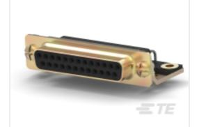
TE Part #5748989-1 D-Sub Receptacle Assembly: Right Angle, Shell Size 3, 2.77mm
