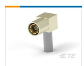
TE Part #413985-1 SMB Connector: Female (Plug), Mated Outer Dia. 4.75mm, 50 Ohm
