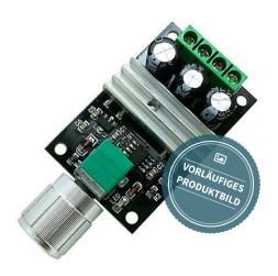
This PWM motor controller allows you to easily and smoothly regulate the rotation speed of your motor. Input and output are provided with convenient screw terminals so that the power supply and motor can be easily connected to the controller.
