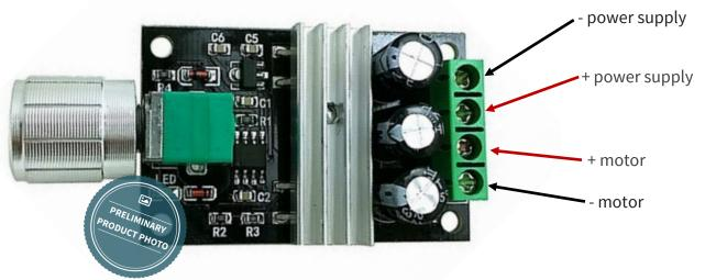
By turning the potentiometer, the speed of the motor is adjusted by PWM.
