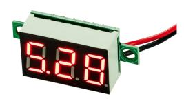
This small mini voltmeter for voltages from 3 to 30 V has a 3 digit 7-segment display (0.36 Inch). The measured value can be displayed with 1 or 2 decimal digits and is refreshed every 0.3 seconds. This measurement device is outstanding by its very low power consumption of less then 30 mA and can be mounted using the 2 mounting holes.
