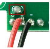
Now you have a new pin assignment on the measuring device. Please note that two ground connections must be connected to the negative terminal of the measuring device (black cable) (one for the measuring voltage and one for the supply voltage).
