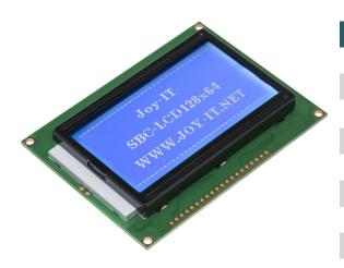
This 128 x 64 graphic LCD is versatile and can be controlled with 8 pin parallel as well as serial via SPI. Its large high-contrast display is suitable for many different applications. The contrast can be adjusted via a potentiometer on the back.
