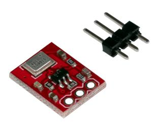
This tiny breakout board features the ADMP401 MEMS microphone. One of the key advantages of this breakout and microphone is the bottom ported input. This means the microphone's input can fit flush against the enclosure of your project.
