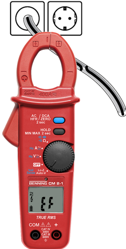
Figure 14: Non-contact phase testing
