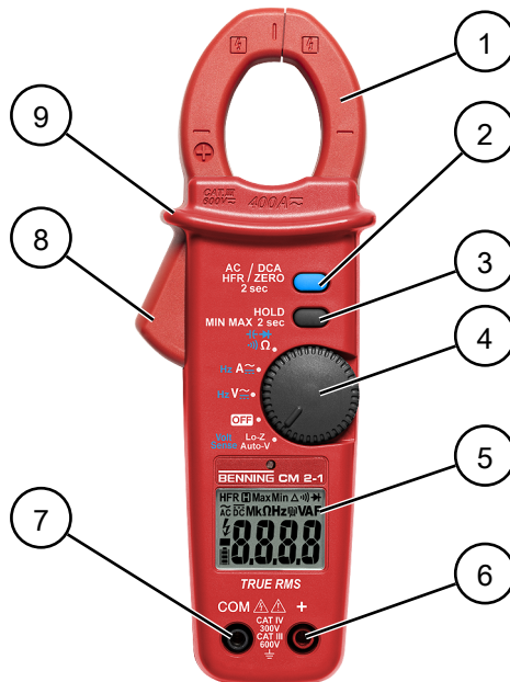
Figure 6: BENNING CM 2-1 device structure
