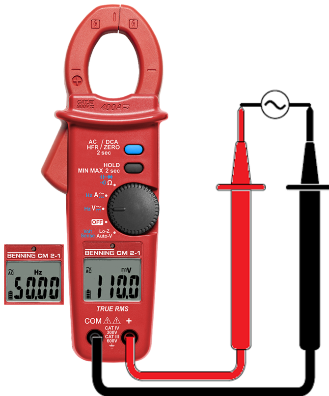
Figure 10: AC voltage or frequency measurement
