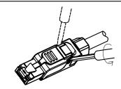
Step 2: Insert the slotted screwdriver into the slot and rotate to open the jaws.
