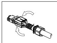
**Step 4 :** Press wiring management to terminate wires.
