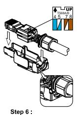
Assemble the wiring management("UP" on the top surface) into the groove of base housing, and locate the nut in the indicated slot.
