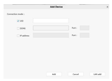
Check DDNS from the Connection Mode. Enter the DDNS and Port of the NVR. Select NVR from the Device types.
