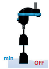
Low level stops the pump
