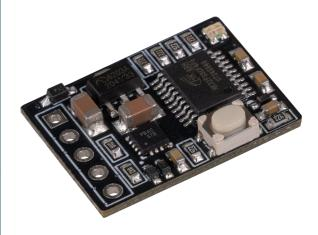
With this small module, you can trigger USB PowerDelivery protocols and thus, for example, charge your laptop via a PD-capable USB-C power supply unit. The output voltage can be adjusted in 5 steps (5 V, 9 V, 12 V, 15 V and 20 V) via the button integrated on the module as well as via the trigger input. The currently selected voltage can be read from the colour of the RGB LED integrated on the module. Due to its interfaces and design, the module can be used flexibly and is highly integrable.
