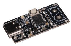
With this small module, you can trigger USB-PD protocols and thus, for example, charge your laptop via a PD-capable USB-C power supply. The output voltage can be adjusted in 5 steps (5 V, 9 V, 12 V, 15 V and 20 V) via the button integrated on the module. The currently selected voltage can be read from the colour of the RGB LED integrated on the module. The module can be used flexibly and is highly integrable.
